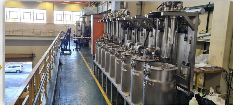
Scale-up to 50 L pilot scale digesters
