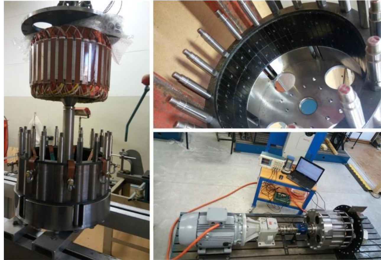
Construction and testing of a 15 kW PMVM
